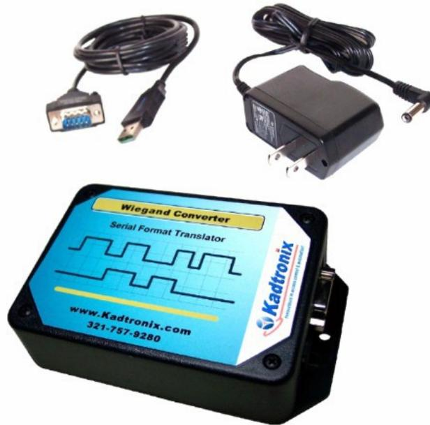
The WRFC is a DCE (data communications equipment) device with DB9 female connector. (Please refer to the applicable note below for additional information.) It also features detachable USB cable and AC adapter. The WRFC is ideally suited for use in access control and other applications where it may be necessary to interface a Wiegand device to a serial host. It provides seamless format conversion, accepting a Wiegand stream of bits and outputting ASCII characters via RS-232.
