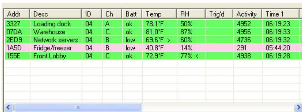
The image shows a table of sensor data. The table has 10 columns: Addr, Desc, ID, Ch, Batt, Temp, RH, Trig'd, Activity, and Time 1. The rows are color-coded: green for recent data and pink for old data. The row for address 1A5D is pink, indicating it is old data.
