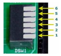
Switches may be adjusted using a miniature screwdriver or similar implement. Available parameter settings are listed below:
