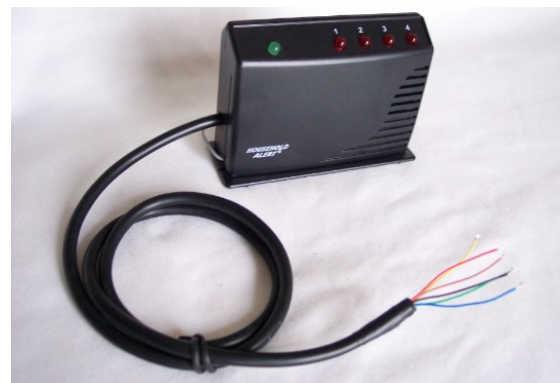
Completed receiver customizations with attached interface cable
