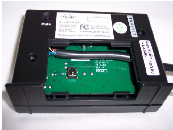
Rear cover reattached (access panel removed, exposing the interface cable)
