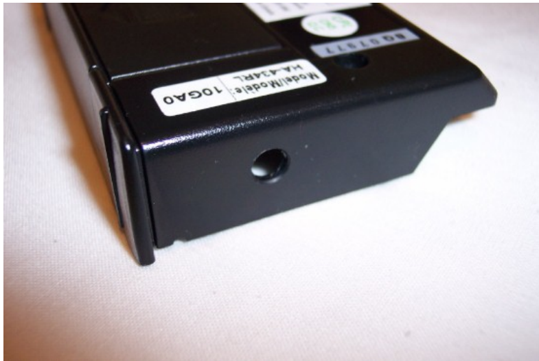
Rear cover with 1/4" cable-entry hole
