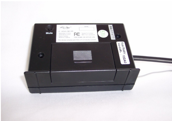
Completed receiver customizations with reattached access panel
