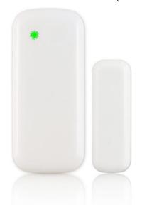
The KD-DS-5800-MINI is suitable for use with a variety of door and window types. Powered by a single CR2032 battery (included), the device provides consistent and reliable sensing with wireless RF signaling. It is a two-part design solution that consists of electronic sensor/transmitter unit and magnet. The device emits RF message signals when the corresponding door or window is opened or closed. (It also sends periodic status updates every 70 to 90 minutes.)
