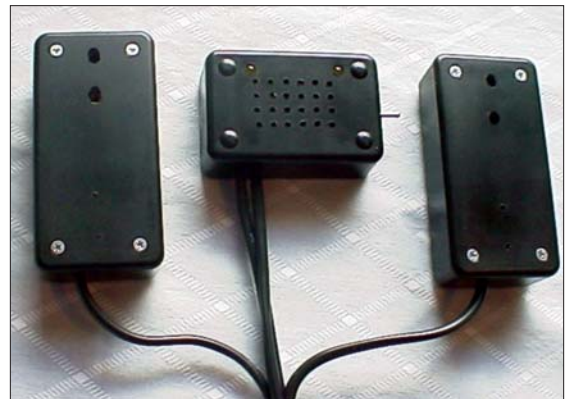
Figure 1: LaneAlert — lane detection system including computer module (center) and two sensor modules (left and right).
