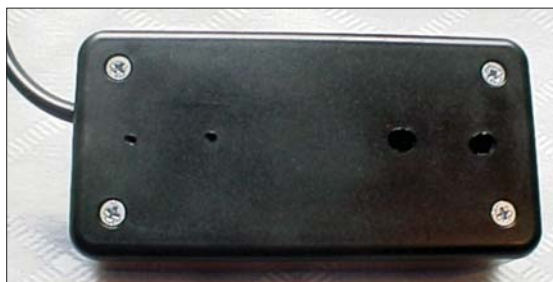
Figure 2: Sensor module — underside view showing cover and four aperture holes.
