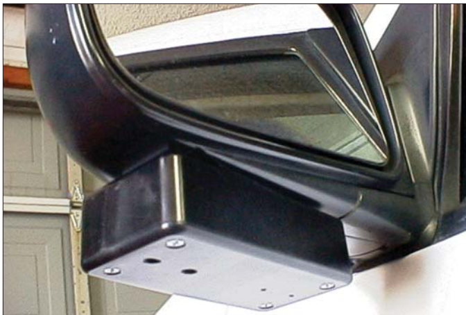
Figure 7: Sensor modules attached to the bottom of the side-view mirror with aperture openings facing down.
