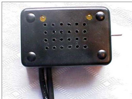
Figure 4: Computer module has two indicator LEDs. Small holes are drilled for the piezo alarm.
