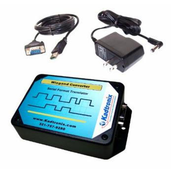
The RWFC is a DCE (data communications equipment) device with DB9 female connector. (Please refer to the applicable note below for additional information.) It also features detachable USB cable and AC adapter. The RWFC is ideally suited for use in access control and other applications where it may be necessary to interface a serial device to a Wiegand-based system. It provides seamless format conversion, accepting a RS-232 source input and outputting a Wiegand stream of bits.
