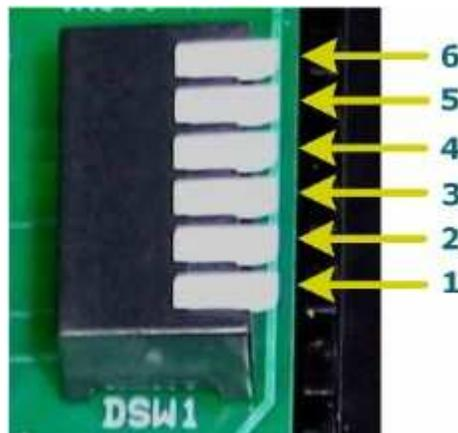
Switches may be adjusted using a miniature screwdriver or similar implement. Available parameter settings are listed below:
