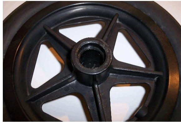
Opposite side: bearing removed, exposing an open hub
